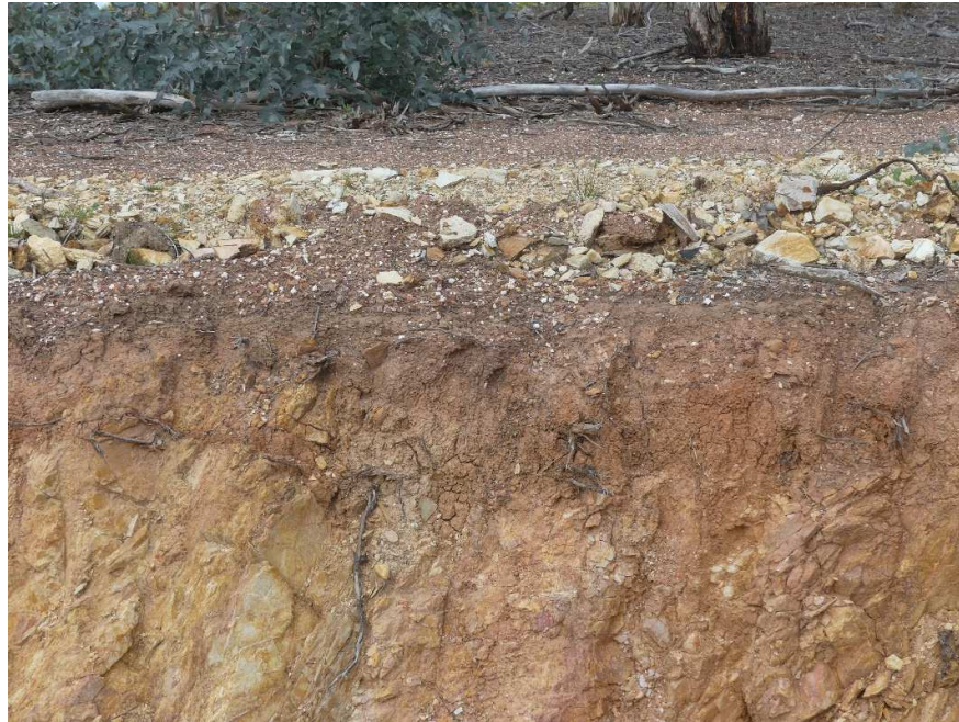
Image.8 Site cut showing the thin A Horizon and the red sodosol B Horizon
