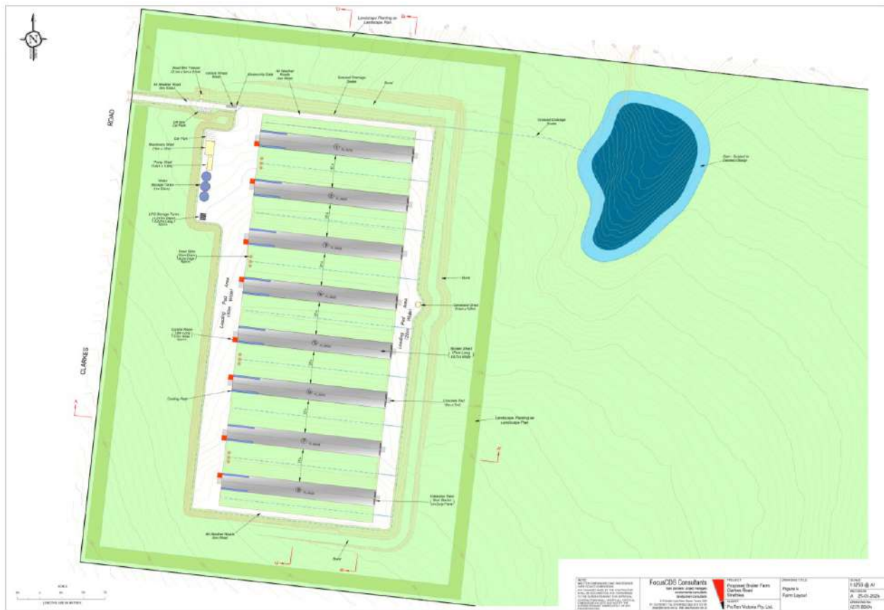
Figure 3-2 Layout of the Proposed Broiler Farm at 141 Clarkes Road Strathlea (FocusCDS Consultants)
