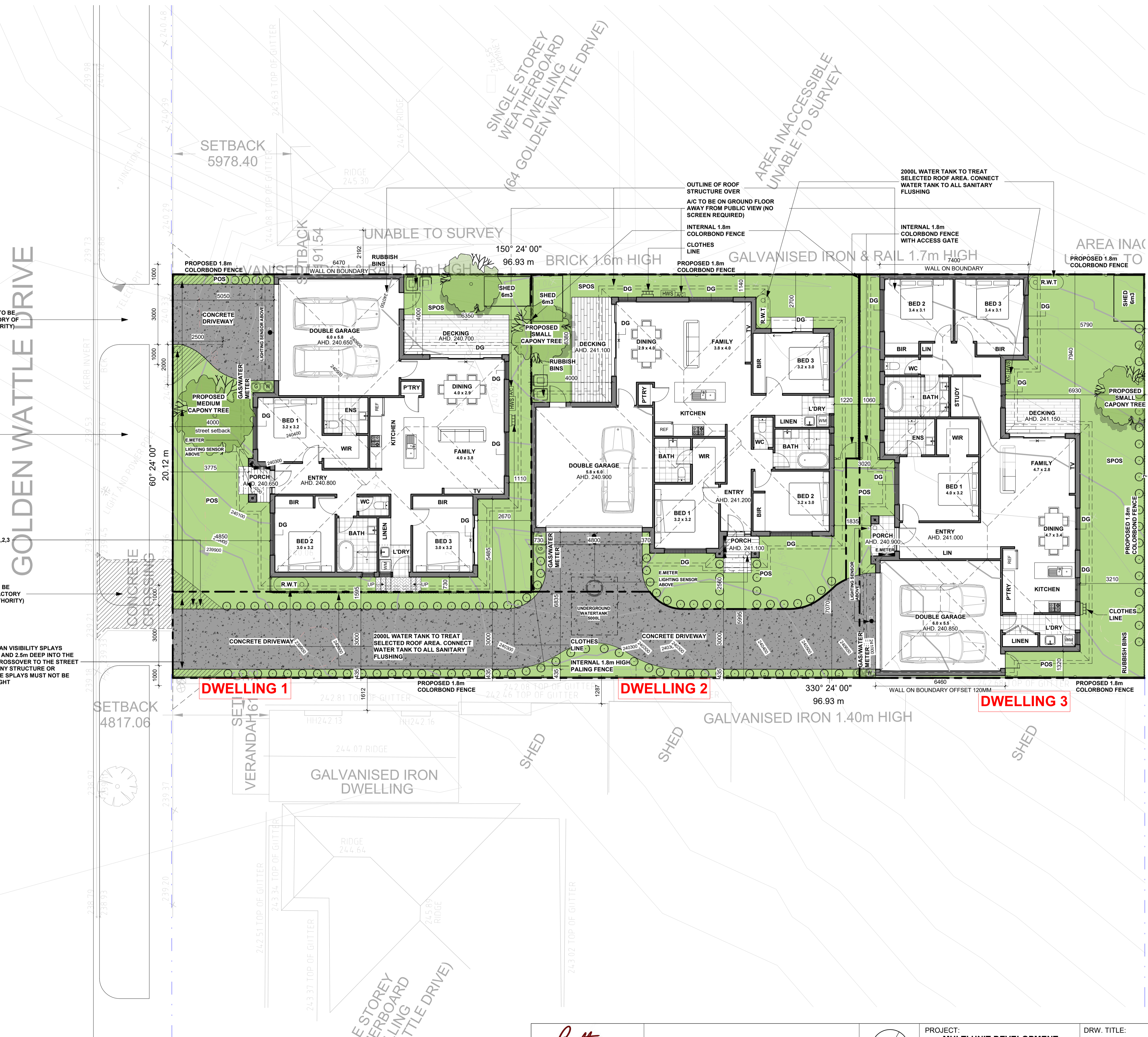
1 GROUND FLOOR PLAN DW 1 - 2 - 3 1 : 100
