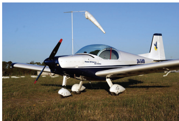
Figure 3-5 - Example of a "3-Axis Aircraft"
