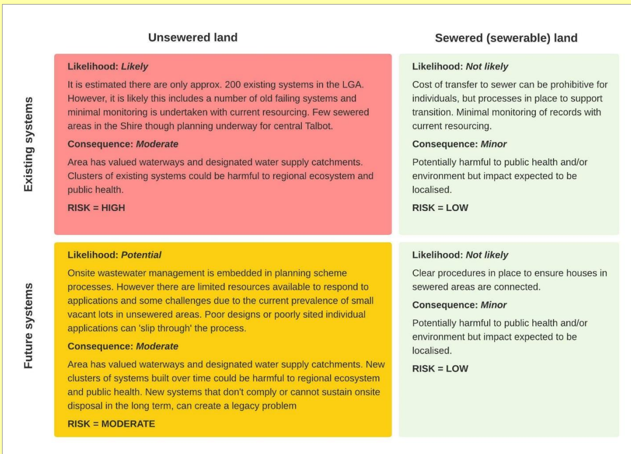
Figure 3-1: Level of risk associated with four categories of onsite wastewater management.
