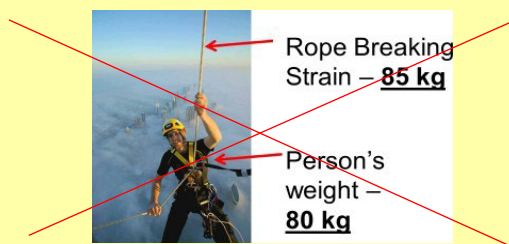
Figure 4-1 Incorrect Factor of Safety
