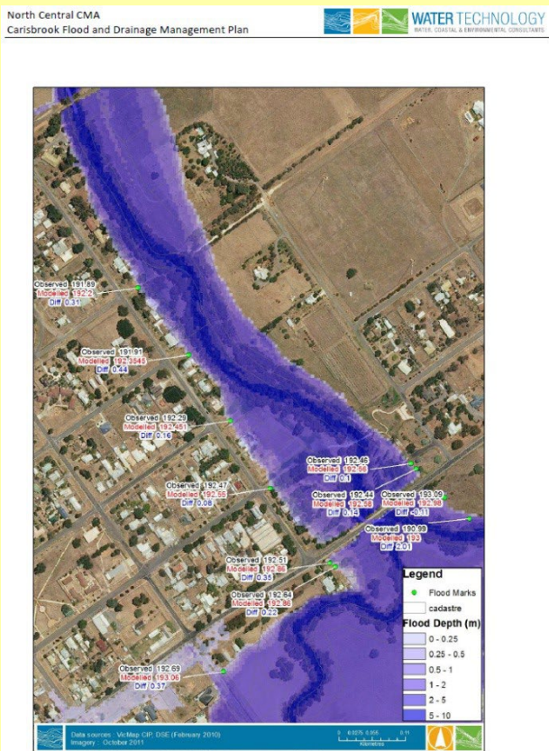
Figure 5-5 Hydraulic model calibration plot – September 2010 (around Pyrenees Hwy bridge)
